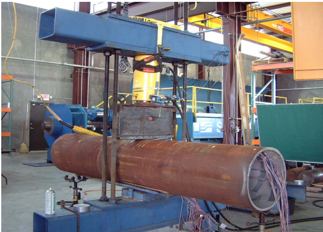
Figure 6 – Photograph of dent installation rig [15]
