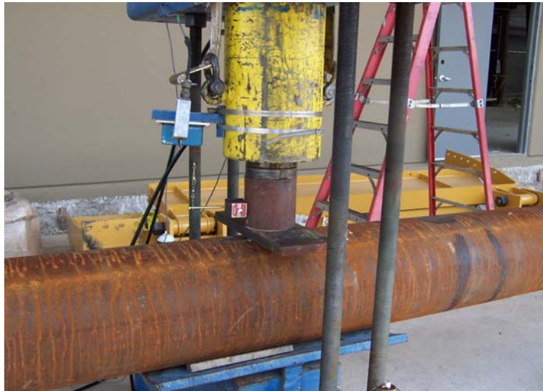
Figure 1 - Dent installation rig to install dents
