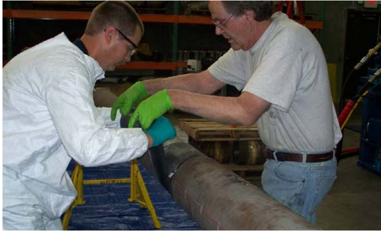
Figure 7 – Installing the hoop wrapped inner carbon layers
