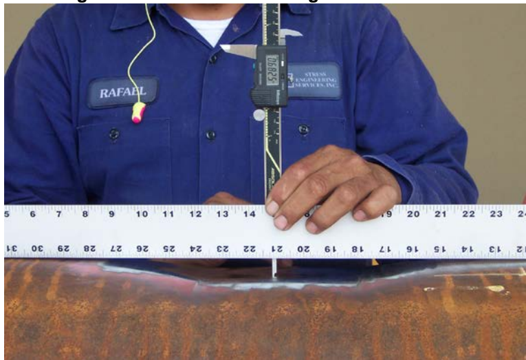
Figure 2 - Measuring dent depth and profile
