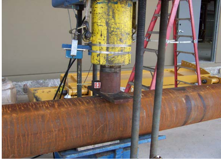
Figure 1 - Dent installation rig to install dents
