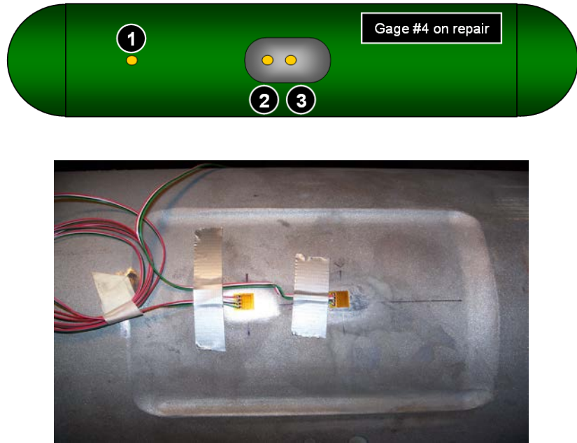
Figure 3 – Schematic showing location of strain gages of photo of machined region
